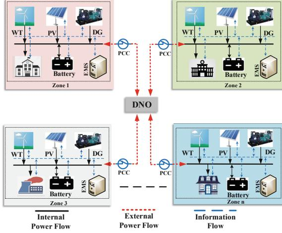
Fig. 1. General representation of Zonal Multi-microgrids structure
