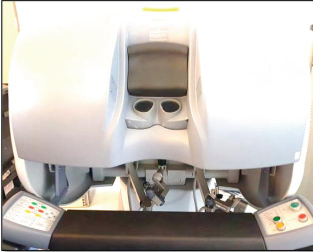
**Fig. 4.** The DVRKT HRSV console and master manipulators.
