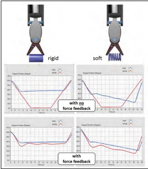
**Fig. 9.** Force-feedback tele-operation of the MTM and PSM Gripper (red and blue lines, respectively): positions *with* and *without* force feedback (top and bottom panels) for rigid and soft objects (left and right panels) are reported. (Color figure online)
