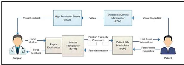
**Fig. 2.** Information flow in RMIS with haptic feedback.
