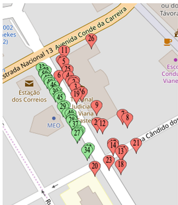
Fig. 2. Correct position vs. received GPS position without any correction (Color figure online)
