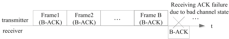
Fig. 4. Receiving ACK failure due to bad channel state.
