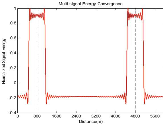
Fig. 11. Interference in specific area with width of 600 m
