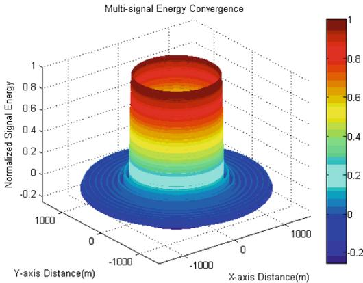
**Fig. 7.** The three-dimensional figure of energy convergence with 16 equal interval frequency wavelets
