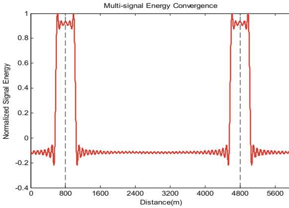
Fig. 10. Interference in specific area with width of 400 m
