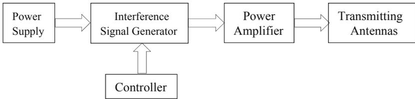
Fig. 1. Structure of the distributed jammer
