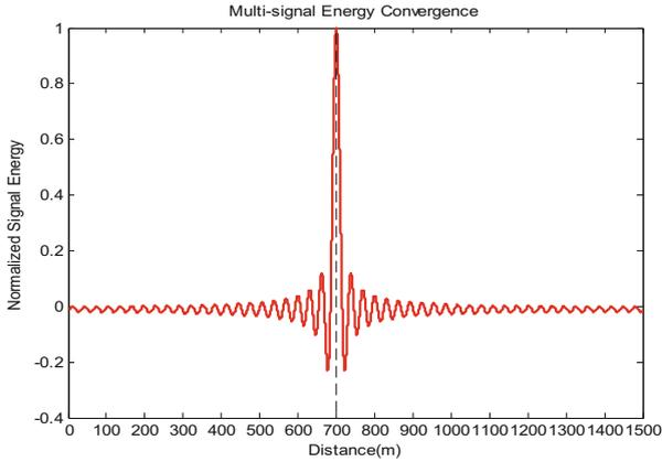
**Fig. 8.** The one-dimensional figure of energy convergence with 48 equal interval frequency wavelets
