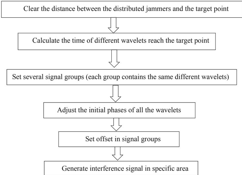
**Fig. 5.** The process of interference generated in the specific area
