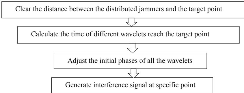
**Fig. 4.** The process of interference generated at the specific point
