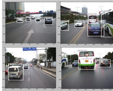
Fig. 5. Testing results of multi-label vehicle detection network.
