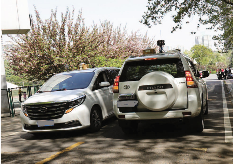
Fig. 1. Vehicles used for measurement: the van on the left side was used for transmitter and the car on the right hand side was used for receiver.
