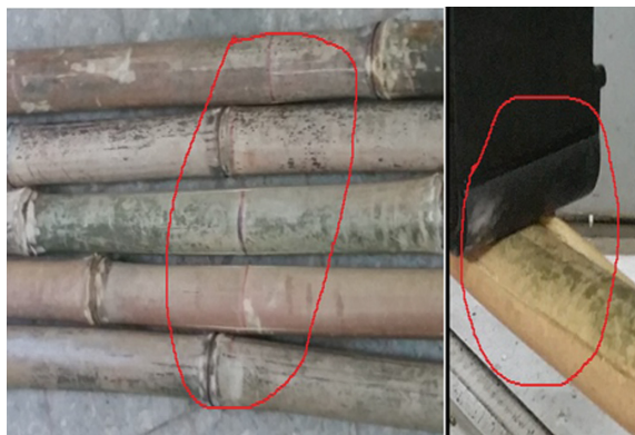
Fig. 8. Hollow bamboo specimen failure during bending test
