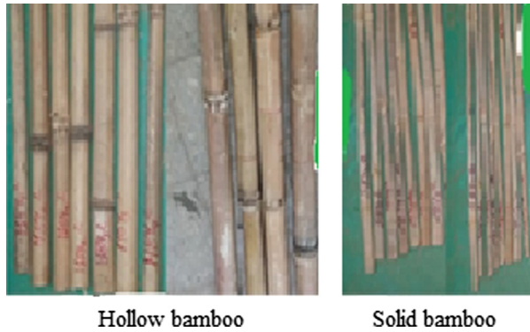
Fig. 7. Bamboo specimens ready for bending test [Photo by the authors]
