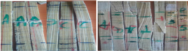
Fig. 15. Bending and tensile samples after failure
