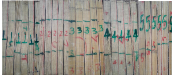
Fig. 5. Samples for tensile test
