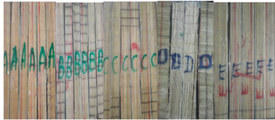
Fig. 6. Samples for bending test according ASTM D-790
