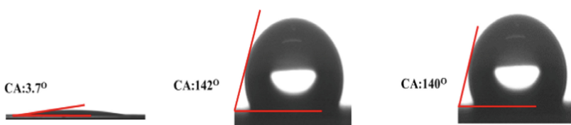
Fig. 7. Chemical stability tests of the grafted membranes (45% metakaolin @ 1200 °C)
