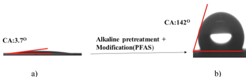
Fig. 6. The water contact angle of the membrane surface: (a) before grafting and (b) after grafting
