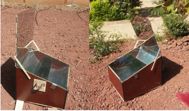
Fig. 6. Constructed Prototype of the solar baking oven (length is reduced for test only)
