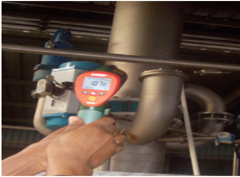
Fig. 1. Infrared temperature measurement taken on wort kettle
