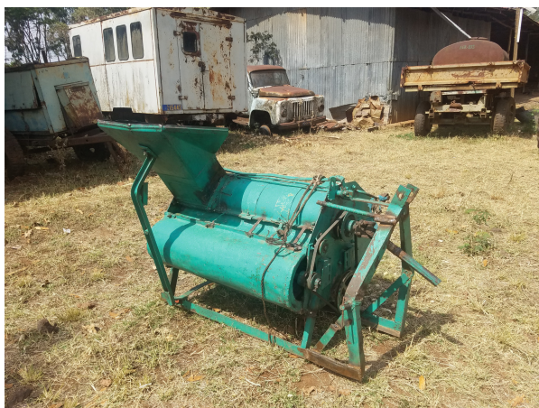
Fig. 4. Sample maize thresher manufactured locally at higher cost than imported ones having low productivity and heavy to transport. (Source: survey result)
