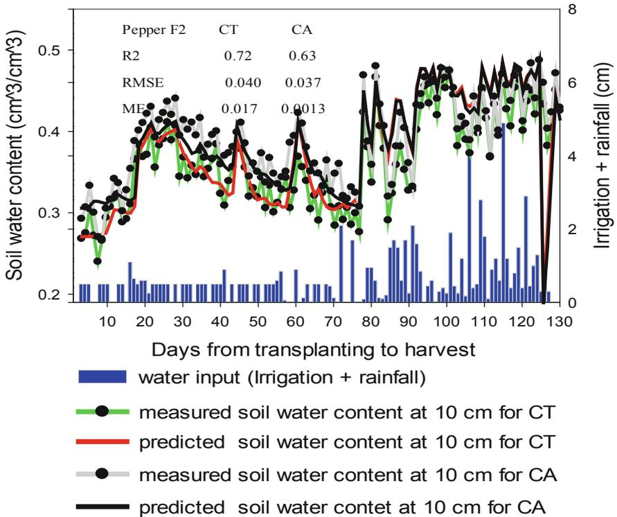
Fig. 4. Comparison of observed and simulated soil water content for CT and CA
