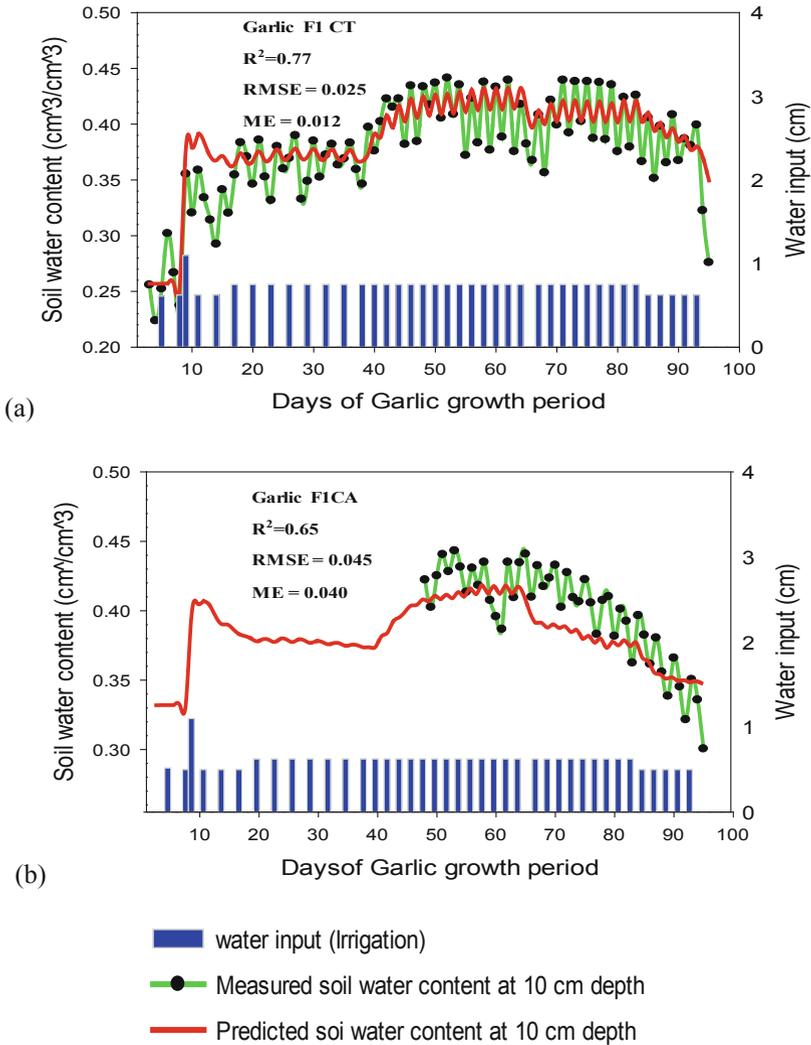
**Fig. 3.** Comparison of observed and simulated soil water content for CT and CA
