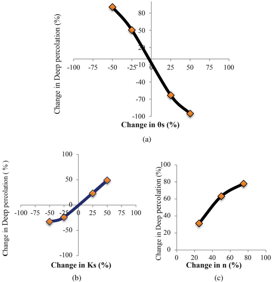
**Fig. 2.** Sensitivity analysis of saturated water content ( $\theta_s$ ) (A), saturated hydraulic conductivity ( $K_s$ ) (B), and pore size distribution parameter (C).
