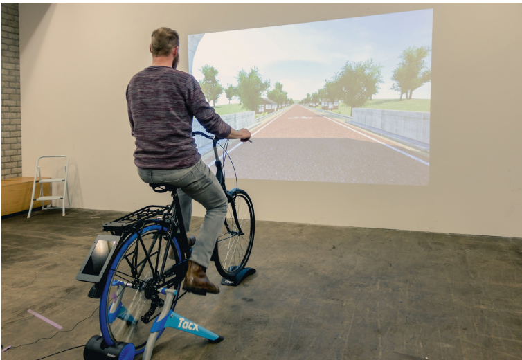
Fig. 5. Cycling simulation system in test.
