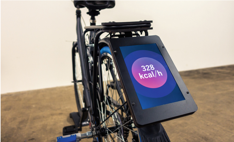
Fig. 2. Prototype of SocialBike’s on-bike display.
