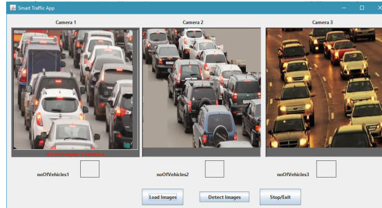
Fig. 7. Smart traffic management system with images loaded
