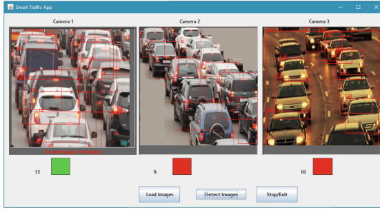
Fig. 8. Smart traffic management system with vehicle detection (Color figure online)
