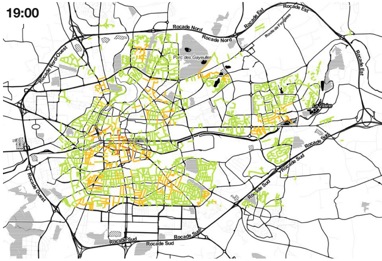
Fig. 4. Predicted on-street parking occupancies in Rennes, France for 7 p.m. in weekdays. Higher occupancy levels are represented with redder hue and lower occupancy levels are represented with greener hue. (Color figure online)
