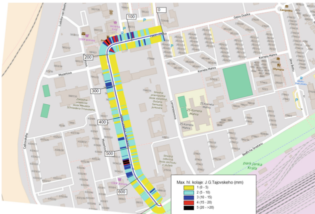
Fig. 6. Evaluation of experimental measurement - depth of track depth.
