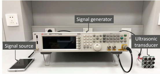
Fig. 10. Experimental setup. A smartphone is used as a signal source, and the signal generator does AM modulation. The modulated signal is transmitted via an array of 9 ultrasonic transducers [15].
