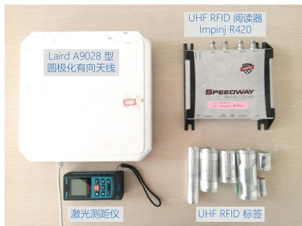
Fig. 7. System main hardware
