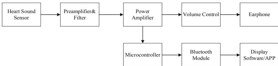
**Fig. 1.** Schematic block diagram of the heart sound sensing system
