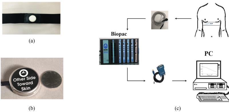
**Fig. 9.** Diagram of the acquisition system ((a) chest strap with piezoelectric sensor (b) TSD108 sensor (c) acquisition system)
