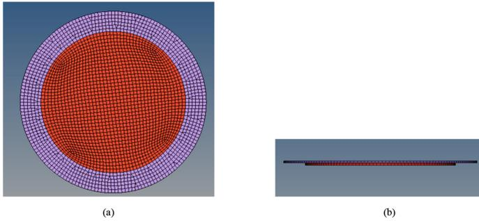
**Fig. 3.** Mesh model of the piezoelectric model (a) vertical view (b) front view
