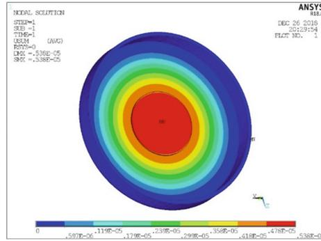
**Fig. 6.** Deformation diagram of piezoelectric sensor (Color figure online)
