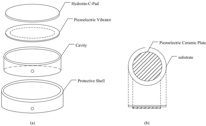
**Fig. 2.** Structure diagram of the piezoelectric sensor ((a) overall structure (b) piezoelectric vibrator structure)
