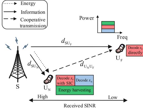
**Fig. 1.** Downlink two-user cooperative NOMA system model, which consists of a base station denoted by S and two paired users denoted by  $U_N$  and  $U_F$ . SIC is performed at  $U_N$  to decode  $x_N$ .
