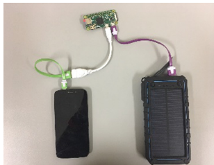
Fig. 1. Showing the bus sensor configuration comprising a Raspberry Pi Zero, 16750 mAh power bank and BLUE LIFE PLAY 2 with a damaged screen
