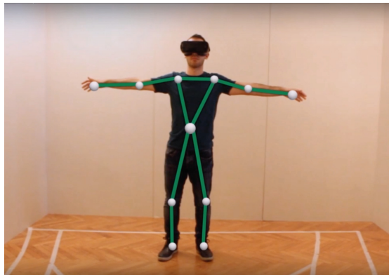
Fig. 1. The MRC is installed in front of the user to recognize the joints and place them inside the virtual environment.
