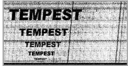
Fig. 6. Test message recovery for Samsung J5, on the 31 MHz reception frequency
