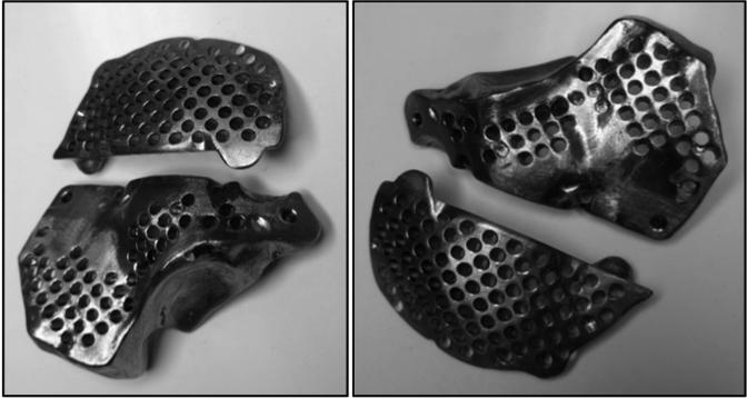
**Fig. 16.** The two pieces of the implant after finishing procedures.
