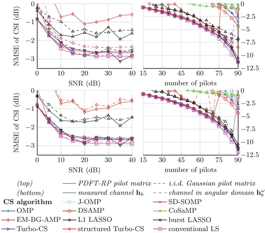
**Fig. 5.** NMSE of CSI in decibels versus SNR (left,  $M = 45$ ) and number of pilot signals  $M$  (right, SNR = 20 dB) of analyzed algorithms depending on pilot matrix (top, averaged for indoor LOS) and channel representation (bottom, averaged for indoor NLOS and static outdoor environments) at 2.4 GHz.
