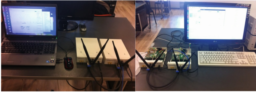
Fig. 7. Transmission and Reception 2 × 2 MIMO
