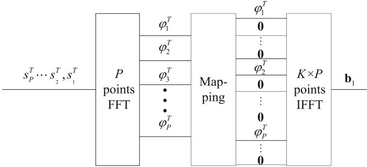
Fig. 3. Pilot design diagram.
