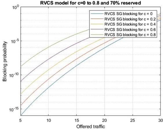
Fig. 9. Blocking probability of RVCS for different 'c'
