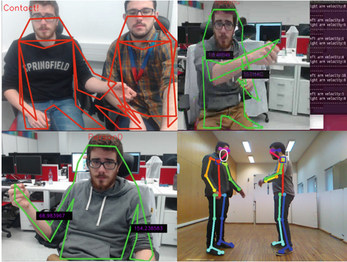
Fig. 2. Examples of the features extracted: contact detection (top left); velocity (top right); angles (bottom left); and tracking (bottom right)
