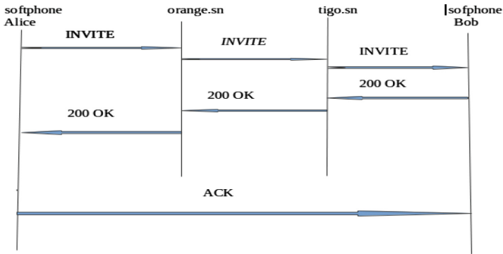
Fig. 4. Session setup between two users who do not have the same provider
