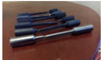
Fig. 5. Tested specimens at fracture point
