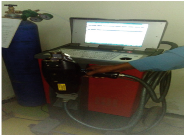
Fig. 1. Spectro test TXC25 machine set up for sample calibrations for CSN 12050 carbon steel experimentation.
