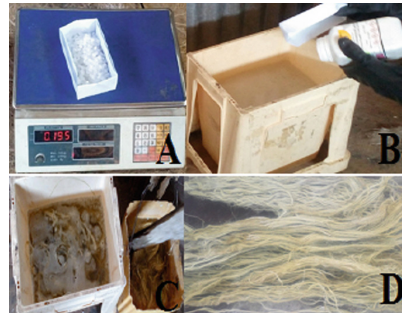
Fig. 1. Alkaline treatment process
