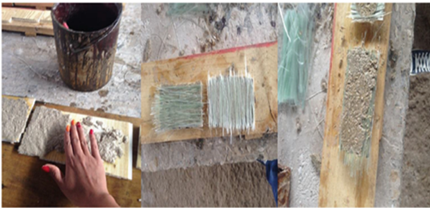
Fig. 4. Hand layup techniques preparation of specimens for testing
