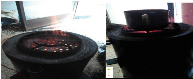
Fig. 4. Testing of manufactured gasifier stove
