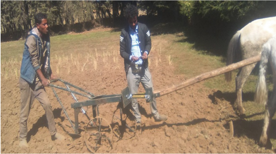
Fig. 20. Multiple mouldboard plough filed performance test setup [Photo by the authors]
