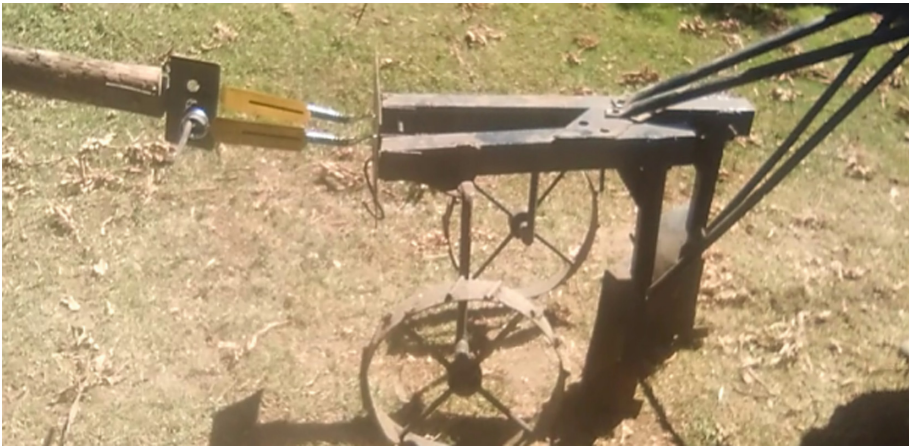
Fig. 18. Multiple mouldboard plough spring dynamometer setup [Photo by the authors]
