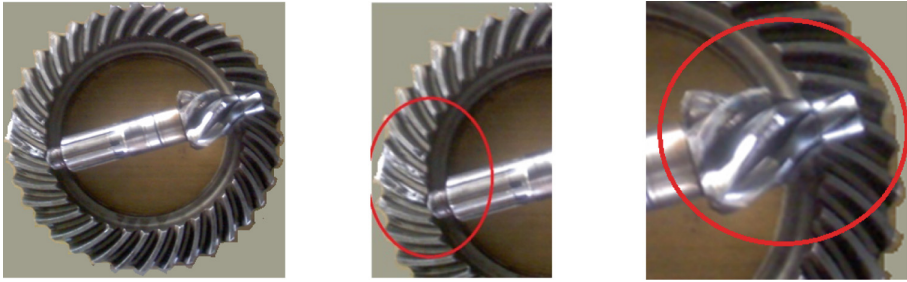
Fig. 1. Failed crown and pinion
