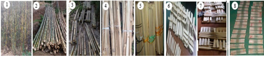
Fig. 3. Steps of specimen preparation for tensile test [Photo by the authors]
