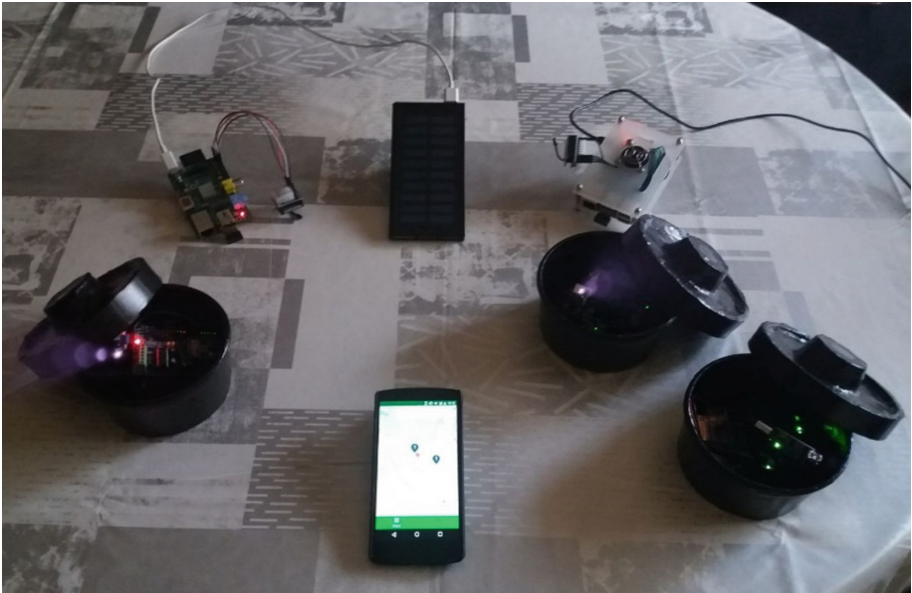
Fig. 6. Complete smart parking prototype test setup.
