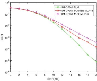
Fig. 4. BER of SM-OFDM-IM system of different detection methods
