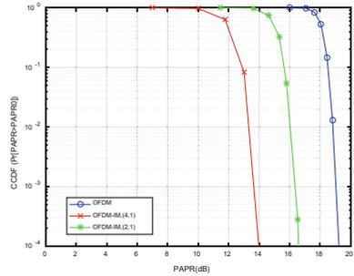
**Fig. 3.** PAPR of OFDM and OFDM-IM systems
