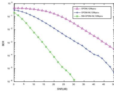
**Fig. 2.** BER of OFDM, OFDM-IM, SM-OFDM-IM systems
