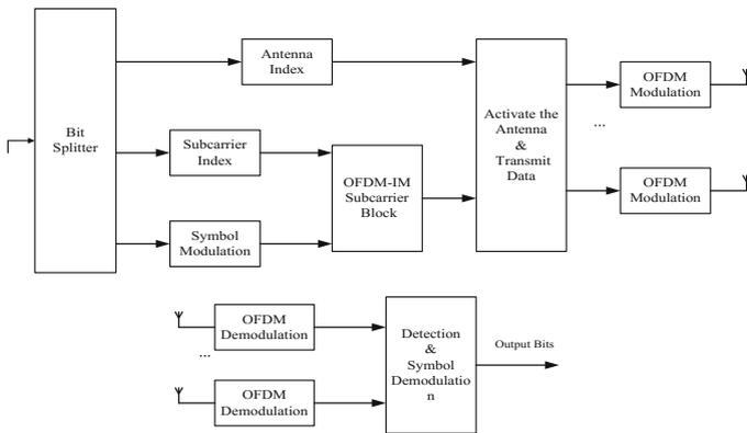
Fig. 1. System model of SM-OFDM-IM
