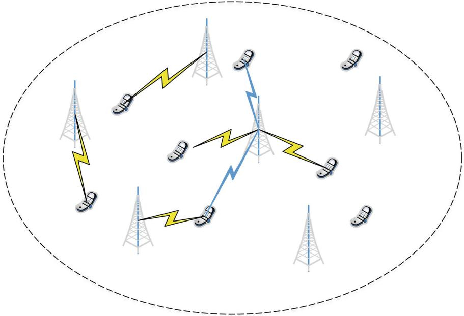
**Fig. 1.** The dense network scenario with  $M$  small-cell BSs and  $K$  users randomly distributed in the circular cell.
