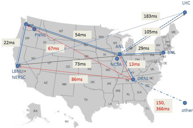
Fig. 3. File transfer infrastructure, showing the six Globus sites and their connections, in blue, plus other connections (in red) considered in emulation studies. The sites are the Argonne Leadership Computing Facility (ALCF) at Argonne National Laboratory (ANL), Brookhaven National Laboratory (BNL), National Energy Research Scientific Computing Center (NERSC) at Lawrence Berkeley National Laboratory (LBNL), Pacific Northwest National Laboratory (PNNL), Oak Ridge Leadership Computing Facility (OLCF) at Oak Ridge National Laboratory (ORNL), and Large Hadron Collider (LHC) at CERN in Europe.
