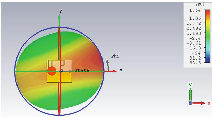
**Fig. 4.** Radiation diagram of the PIFA antenna using the PCB simplified model.
