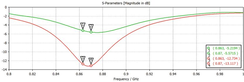
**Fig. 3.**  $S_{11}$ -parameter obtained after simulation. Green line represents the theoretical model and Red line represents the optimized model after multiple adjustments. (Color figure online)
