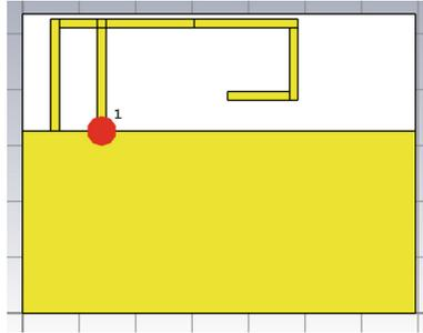
**Fig. 2.** Simulation model with groundplane and the PIFA antenna included.
