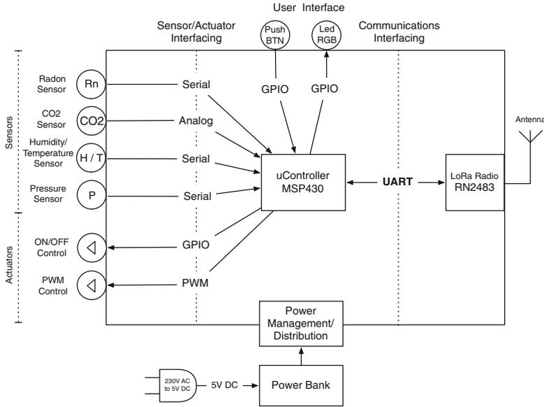
**Fig. 1.** Block diagram of the Compact LoRa Device.
