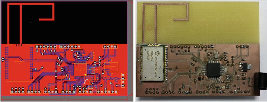
**Fig. 5.** PCB design with antenna and assembled version.
