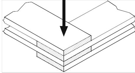
**Fig. 7.** Load applied on the lap joints
