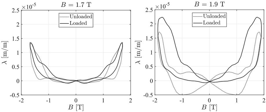
**Fig. 8.** Influence of a clamping load applied on the core joints.
