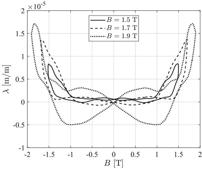
**Fig. 6.** Magnetostriction as a function of the magnetic polarization (13 strips per limb).
