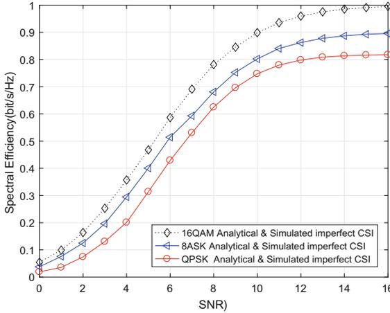
**Fig. 4.** Spectral efficiency for various Modulation schemes
