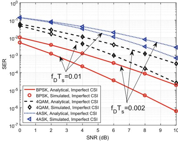
**Fig. 2.** The analytical and simulated SER as a function of SNR.
