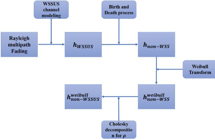
Fig. 2. Model structure for the proposed non-WSSUS V2V channel model.
