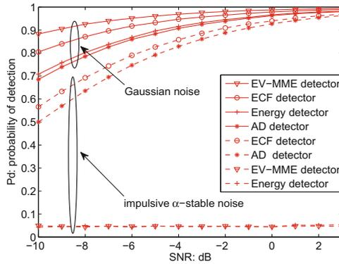
**Fig. 3.** Detection performance comparison among the proposed ECF detector, energy detector, EV-MME detector and AD detector under Gaussian noise and impulsive noise, with parameters  $\gamma = 1, \alpha = 1.5$ , with  $N_0 = 500$  noise-only samples and  $N = 500$  observations, 16-QAM modulated signal
