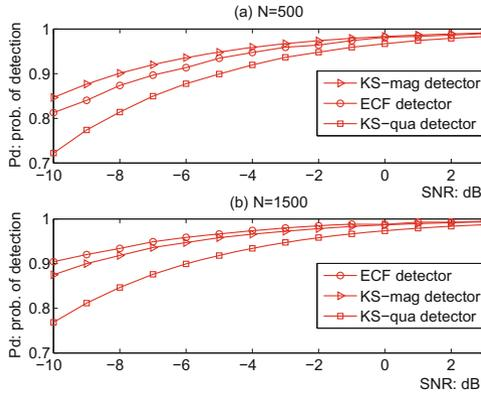
**Fig. 4.** Detection performance comparison between the proposed ECF detector and KS detector with  $N_0 = 500$  independent noise-only samples under Gaussian noise environment. Observation samples: (a)  $N = 500$ , (b)  $N = 1500$
