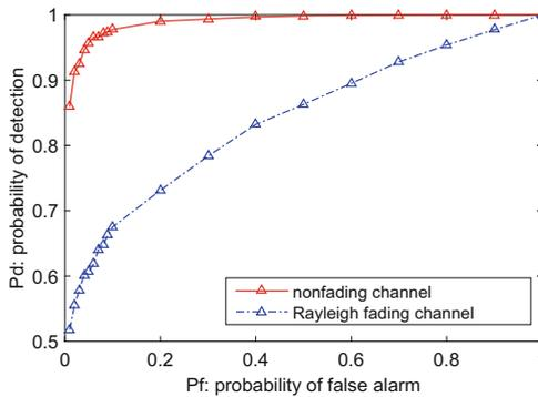
**Fig. 1.** ROC curves of the proposed ECF detector over nonfading and Rayleigh fading channel, with  $N_0 = 500$  noise-only samples and  $N = 500$  observations, the average SNR is  $-9dB$ , impulsive noise parameters  $\gamma = 1, \alpha = 1.5$
