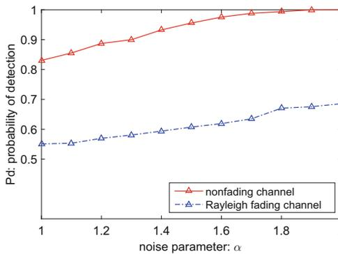
**Fig. 2.** Detection probability of the ECF detector versus noise parameter  $\alpha$  over non-fading and Rayleigh fading channel, with  $\gamma = 1, N_0 = 500$  noise-only samples and  $N = 500$  observations,  $P_f = 0.05$ , SNR  $= -9dB$ , 16-QAM modulated signal.
