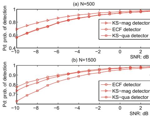
**Fig. 5.** Detection performance comparison between the proposed ECF detector and KS detector under impulsive noise environment, with  $N_0 = 500$  independent noise-only samples, (a)  $N = 500$ , (b)  $N = 1500$  observation samples, impulsive noise parameters are  $\gamma = 1, \alpha = 1.5$ .
