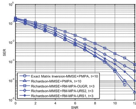
Fig. 3. SER performance comparison of two stages detections
