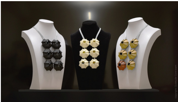
Fig. 3. 3D shape-change fabric modules (left), felt necklace with light patterns (center), regenerated leather necklace with vibration (right).
